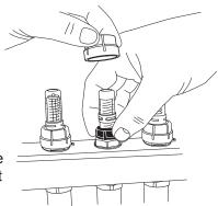
Do not twist the glass as this will completely remove the gauge, this is designed only to be removed for cleaning purposes, and when the flow has been isolated.
