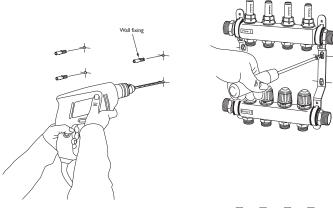
Make sure that the manifold is level and that it is high enough so that the pipes can be installed easily.
