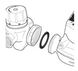
Connect the Thermoguard UFH valve to the pump using the pump nut which is pre-assembled to the Thermoguard, ensuring the pump washer is inserted. Please take note of the directional arrow on the pump body.
