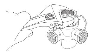
Slide the piston/thermostat assembly and spring out of the valve body.
