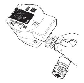
Connect the nickel plated elbow to the pump using the 1 ½" pump nut, ensuring the pump washer is inserted.
