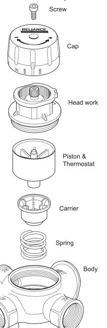
Remove the valve headwork by unscrewing the large plastic hex nut with an adjustable spanner.
